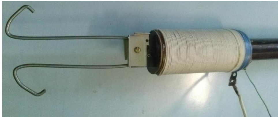
Fig. 6. The induction heater coil appearance.
